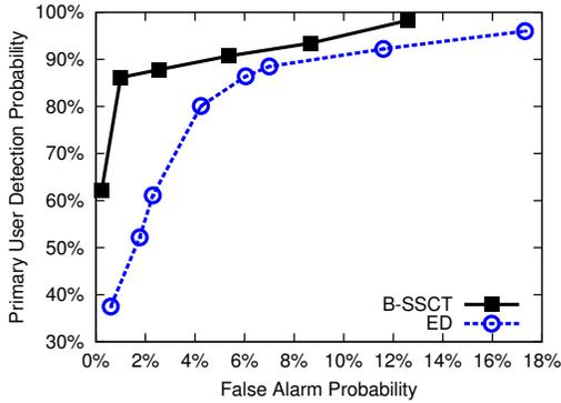
Fig. 6. ROC Performance: B-SSCT versus Energy Detection.
