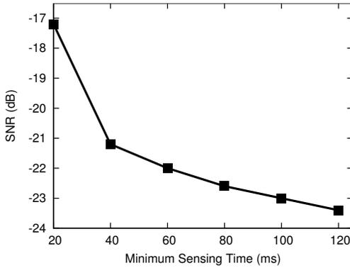
Fig. 1. Minimum required sensing time for energy detection based on experiments.
