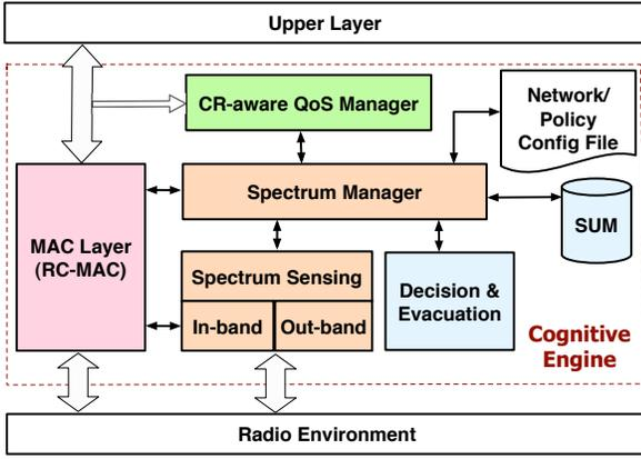
Fig. 3. RECOG system architecture.
