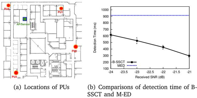
Fig. 8. Detection speed: B-SSCT vs. M-ED
