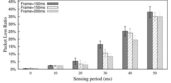
(b) VoIP packet loss ratio vs. length of a sensing period
