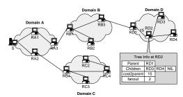
Fig. 2. Logical view of tree topology for (S,G).
