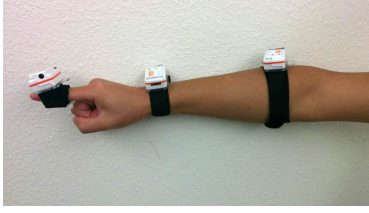
Figure 3: 3 Shimmers used to measure finger, wrist and forearm motion
