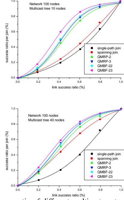
Fig.4. Success ratio of different multicast protocols with two group size
