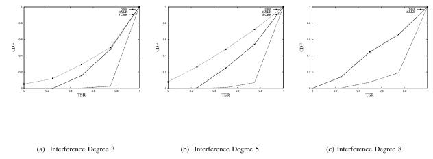
Fig. 1: CDF (percentage of femtocells) of throughput satisfaction rate in small-sized femtocell networks
