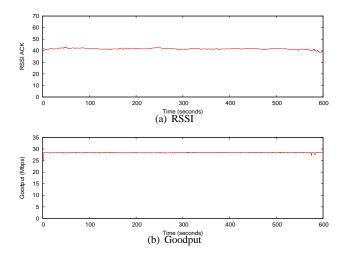
Fig. 3. Single Link at 54Mbps Modulation Rate
