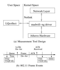
Fig. 1. The Measurement Tool
