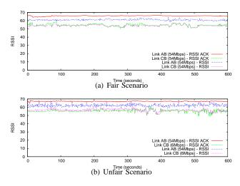
Fig. 6. Inter-Flow Comparison of RSSI and RSSI ACK
