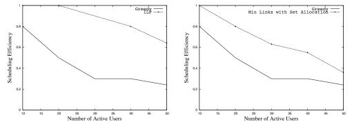
Fig. 2. Performance of ILP and Min Links with Set Allocation (2 antennas)
