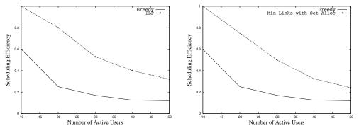
Fig. 1. Performance of ILP and Min Links with Set Allocation (1 antenna)
