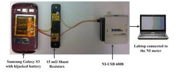
Fig. 1. Power measurement setup
