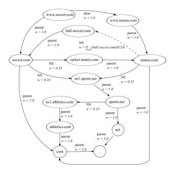
Fig. 2. The dependency graph for the domain name *www.soccer.com*, derived from the zone data in Table I. The solid lines represent active influence, and the dashed lines represent passive influence.
