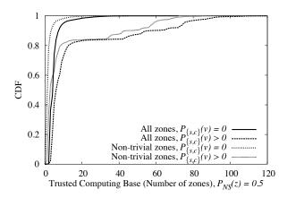
Fig. 4. The CDF for the size of the TCB of ODP/SC08 hostnames. Included are the CDF for the number non-trivial and total zones in the TCB, for  $P_{\{s,c\}}(v) = 0$  and  $P_{\{s,c\}}(v) > 0$ .
