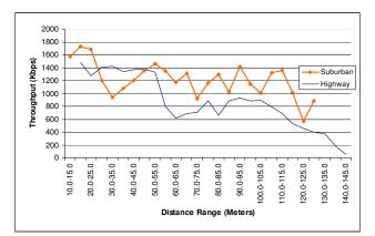
Figure 1. TCP Throughputs vs. Distance
