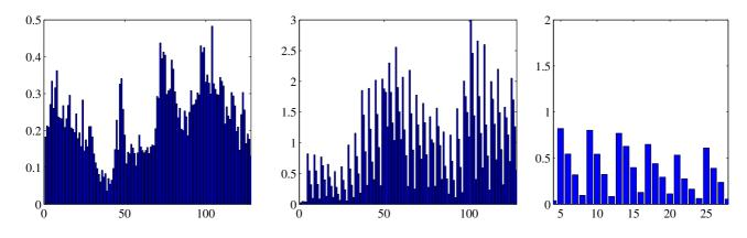
Fig. 3. Sample histogram plot for transform coefficients across rows and columns for diagonal coefficient of wavelet decomposition using orthogonal wavelet for (a-left) original frame, and (b-middle) frame with blocking. (c-right) shows zoom-in to (b) showing clear staircase like pattern with repetition every 4 pixels. The entire sample frame ( $512 \times 512$  pixels) is considered as a single tile for illustration purposes.
