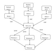
Figure 4. Service differentiation testbed configuration.
