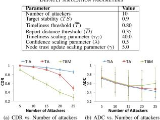
Fig. 3. Performance Comparison of TIA vs. TA vs. TBM in CDR and ADC
