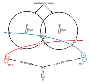
(a) MS trajectory. The letters in the small circles are the time the MS's arrive at that point
