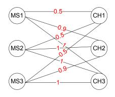
Fig. 2. A bipartite graph with 3 MS's and 3 Channels (CH). The numbers are the weight of the edges.
